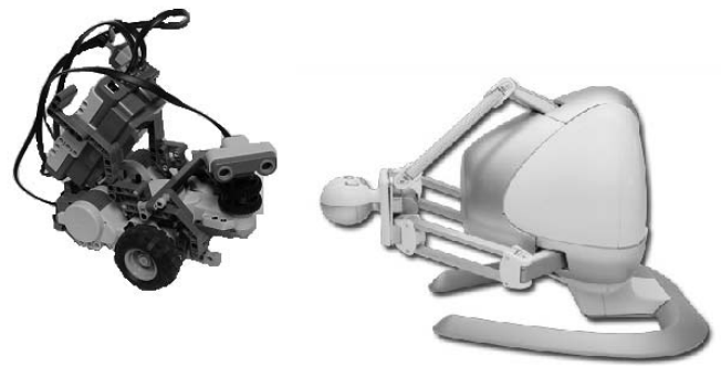
Fig. 9. The LegoNXT mobile robot with rotational sonar sensory system and the Novint Falcon force-feedback haptic interface.
