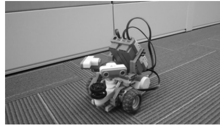
Fig. 3 Lego NXT autonomous mobile robot equipped with two sonar sensors. sources of uncertainty disappear, the uncertainty quantifiers all reduce to zero.
