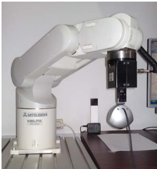
Figure 8. serial robot with mounted camera
