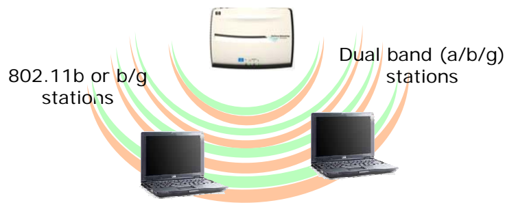
Figure 5. Simultaneous 802.11a and 802.11g dual radio support
