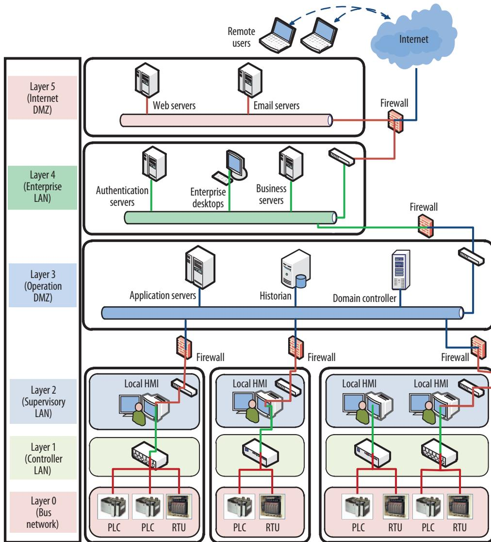
**Figure 2. SCADA system layers. Most forensic analysis involves layers 0-2, which contain the components that control the underlying industrial processes.**
