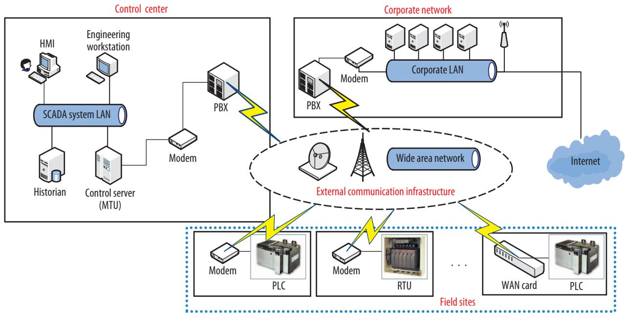
**Figure 1. Simplified logical view of a typical supervisory control and data acquisition (SCADA) architecture.**
