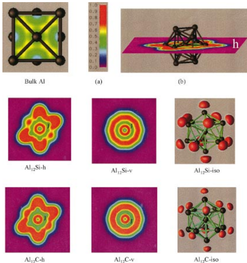
FIG. 1. (Color) Constant electronic charge density surfaces for the excess (a) and depletion (b) of charge in \text{Al}_{12}\text{Si} as compared to the overlapping densities of \text{Al}_{12} and Si atoms, respectively. (c) and (d) are the corresponding constant charge density surfaces for \text{Al}_{12}\text{C} . The values of charge in the four cases (a)–(d) are 0.052, 0.055, 0.038, and 0.048 electrons/ \text{\AA}^3 , respectively. Red color is for charge density and black balls represent ions.
