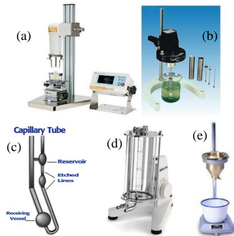
Figure 1. Common viscometers: (a) vibration based [15], (b) rotational [16], (c) capillary [17], (d) falling-ball [18], (e) cup-type [19].
